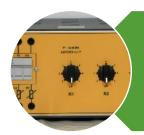
Variable resistive, inductive and capacitive loads simulate the end-users consumption.
